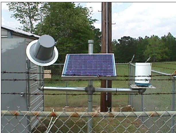
Figure 5-2 Typical Field Installation of Precipitation Gage
